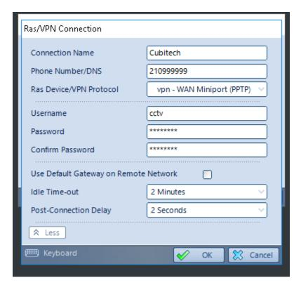
Notes: Cubis server must have an ISDN modem install for this connection type to work properly.
