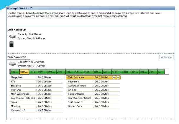
The system can "Auto Size" the available storage for each camera by clicking the "Auto Size" button or you can control the storage for each camera by moving the mouse over the camera list on the bottom of the graph and clicking on "+" for increasing the HDD allocated space for the camera or by clicking on "-" for decreasing it.
